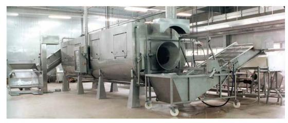
One of the oldest continuous machine types used for classical meat processing and for cooking sausages. The combination KODUKO / KODUKÜ (Continuous cooking and cooling plant) has been manufactured by Berief since the 50s and has been used with great success.
