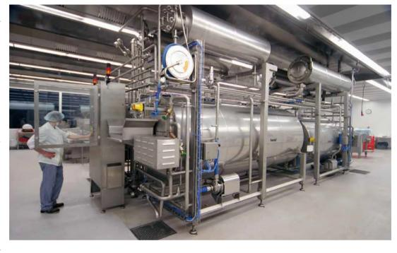
trained staff is required but also a reliable supplier of processing technology. In the field of thermal production of meals, Frankenberg committed the proven roasting and cooking technology from Berief. The rising demands for quality and quantity of the menu components are met with a new twin cooking system. This line is based on the proven technology of the continuous KODUKO / KODUKÜ cooking and cooling systems. Among others, rice and pasta products are cooked and vegetables are blanched in
